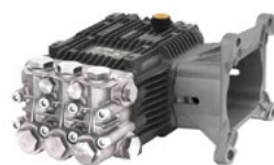
Pompe HP 275 bars 15.1L/mm 3400trs DX HN RKV 4G40 D+F41
