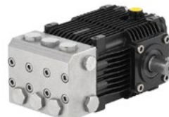
Pompe HP 150 bars 21L/mn 1450trs DX N RK SS 21.5
