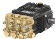
Pompe HP 150 bars 15L/mn 1450 trs DX N RK 15.15
