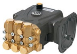
Pompe HP 200 bars 15L/mm 1450 trs DX C RR 15.20+flange type F16
